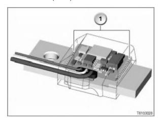
1 Spring element (gull wings) on intelligent battery sensor (IBS)
